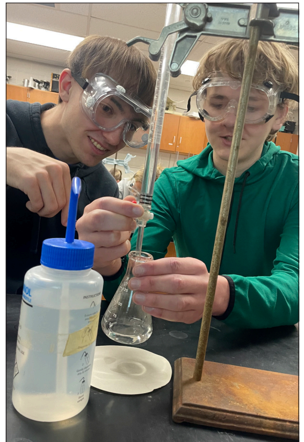
ONTARIO HIGH SCHOOL chemistry students determined the concentration of acid in vinegar via a technique called titration.
